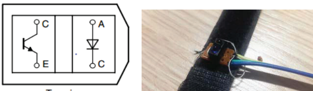
Figure 3. An TCRT5000 sensor is embedded onto a wearable fabric for measuring heartbeat.
