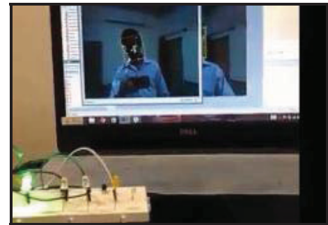
Figure 5. Facial Monitor by Interacting Face Tracking with LEDs using Raspberry Pi in Matlab.
