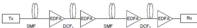
Fig. 1. Traditional setup for dispersion compensation using DCF for 2-spans system. Tx: Transmitter, Rx: Receiver
