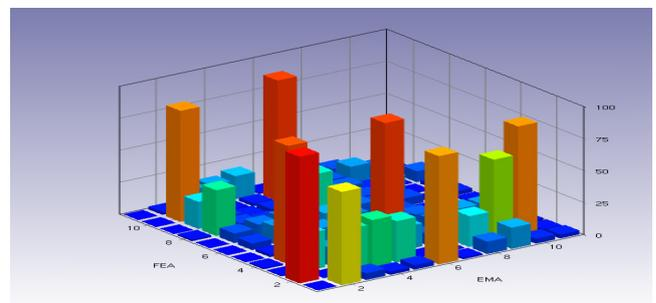
Figure 4. Comparison of 3D plots of MAC matrices to first eleven mode shapes of structure.
