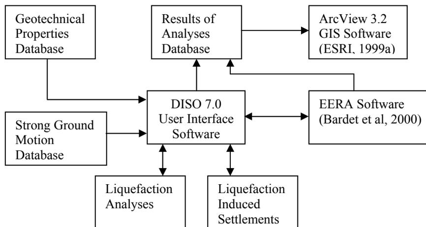
Figure 1. Modular Structure of DISO 7.0 Processing Units
