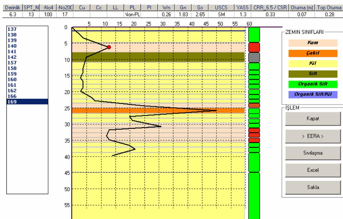
Figure 3. Liquefaction analysis window for Borehole #169 (DISO 7.0 software)
