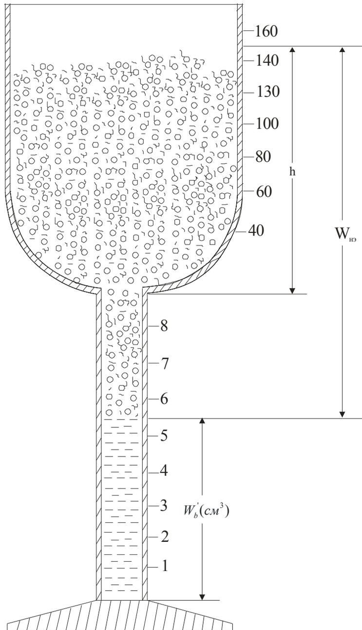
Figure 1. Graduated vessel for sedimentation
