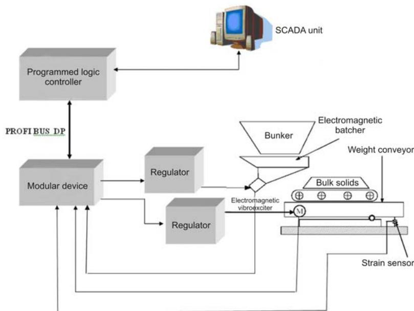
Fig. 1. Control system vibrating injector.
