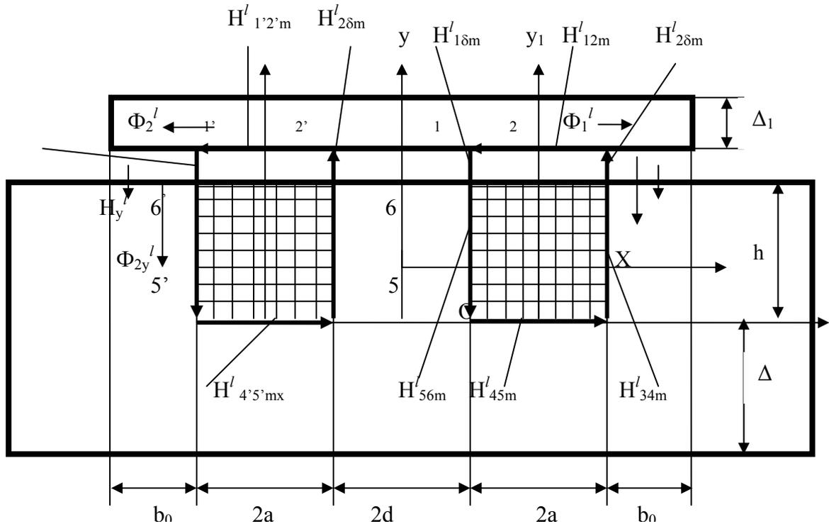
Fig. 1 Magnetic fluxes around TFEMC winding
